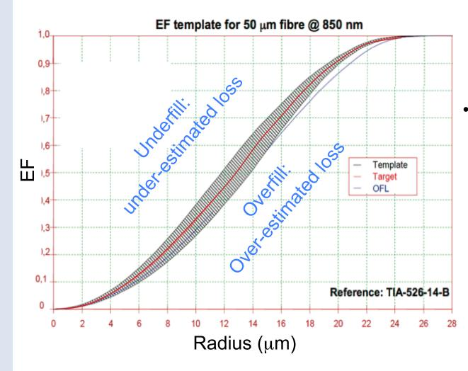
EF within template ensures loss measurements comparable within a given tolerance interval
