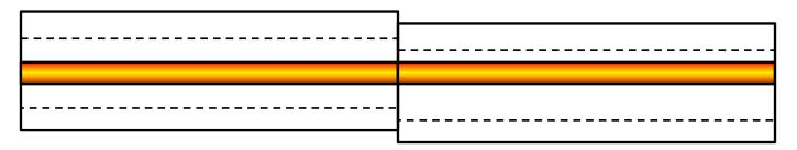
Overfill:large sensitivity of the coupling losses to lateral misalignment
