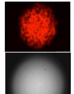
Superposition of all guided modes lead to complex intensity patterns, depending on fibre and source properties
